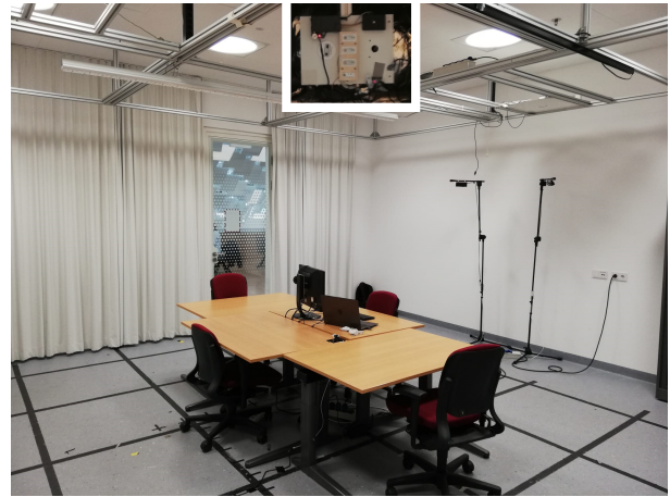
Fig. 13. Experimental setup of indoor space with four workspaces, with a zoomed view of the sensor setup at the ceiling.
