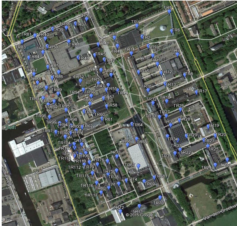
Fig. 2. Candidate radar positions for the TU-Delft campus. The area dimension is approx. 400 000 m 2 .
