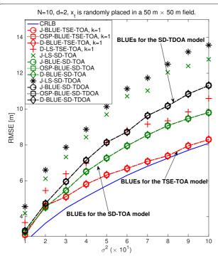
**Fig. 2** Performance of different time-based estimators: the target node is randomly placed in a  $50 \times 50$  field and 10 anchors are deployed with coordinates (50, 50), (50, 0), (0, 50), (0, 0), (25, 7), (25, 43), (12, 33), (12, 16), (37, 33), and (37, 16)
