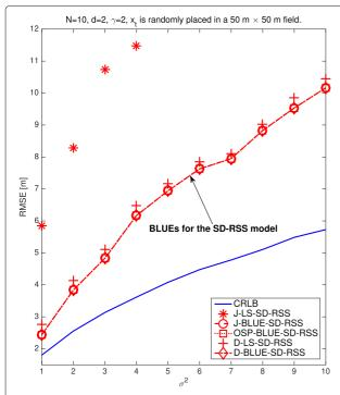
**Fig. 3** Performance of different RSS-based estimators: the target node is randomly placed in a  $50 \times 50$  field and 10 anchors are deployed with coordinates of (50,50), (50,0), (0,50), (0,0), (25,7), (25,43), (12,33), (12,16), (37,33), and (37,16). The transmit power is set to 10 dBm and the PLE is set to 2
