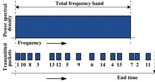
Fig. 3. Sequence of packet transmission in time domain using whole operating bandwidth (single channel scenario).
