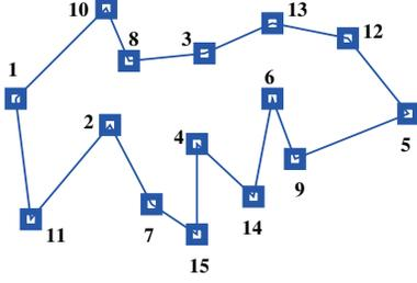
Fig. 2. An example of the Hamiltonian cycle in a network with 15 nodes. The length of the cycle is proportional to the sum of all the propagation delays between transmitting nodes.
