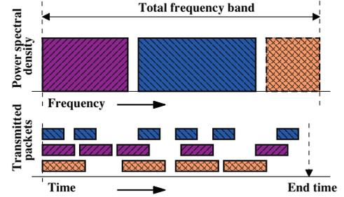
Fig. 5. An example of the parallel transmissions of the packets in time domain from different groups of nodes. The bandwidth allocation in the frequency domain for each group is shown in the upper part of the figure.
