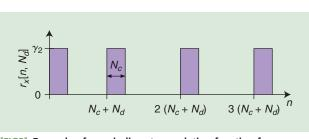
[FIG3] Example of a periodic autocorrelation function for an OFDM signal with a CP.
