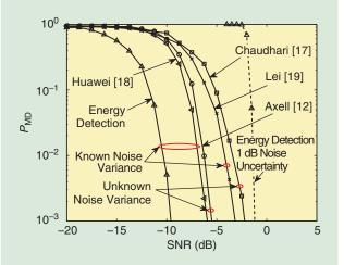
[FIG4] Comparison of the autocorrelation-based detection schemes.  $P_{FA} = 0.05$ ,  $N_d = 32$ ,  $N_c = 8$ , and K = 50.
