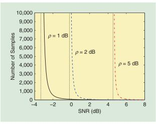
[FIG1] The number of samples required to meet  $P_{FA} = 0.05$  and  $P_D = 0.9$  using energy detection under noise uncertainty.
