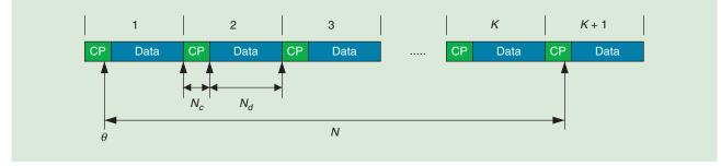
[FIG2] Model for the N samples of a received OFDM signal.
