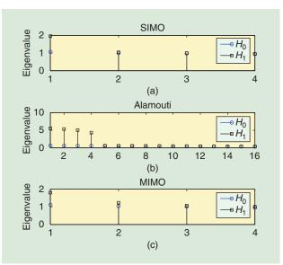
[FIG5] Example of the sorted eigenvalues of the sample covariance matrix  $\hat{R}$  with four receive antennas, for N = 1,000 and SNR =  $10 \log_{10} (\gamma^2 / \sigma^2) = 0$  dB. The Alamouti scheme codes two complex symbols over two time intervals and two antennas.
