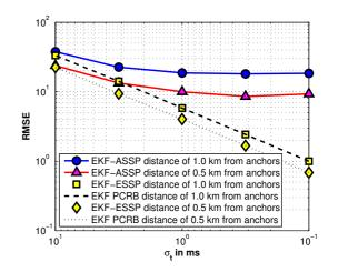
Fig. 5. Effect of the time measurement error on the proposed algorithm.
