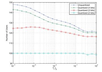
Fig. 4. Average number of users that are scheduled per block for a varying product of block length  $T_{\rm f}$  and Doppler frequency  $f_{\rm D}$ . (M = 2, K = 100, 150 users, 1000 blocks, Q = 30, SNR = 15 dB, SINR<sub>min</sub> = 5 dB).
