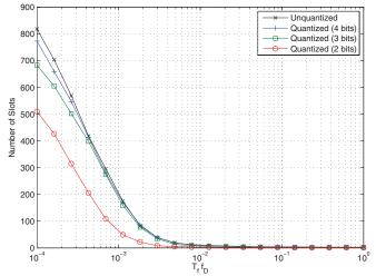
Fig. 3. Average number of slots that a user is successively scheduled for a varying product of block length  $T_{\rm f}$  and Doppler frequency  $f_{\rm D}$ . (M = 2, K = 100, 150 users, 1000 blocks, SNR = 15 dB, SINR<sub>min</sub> = 5 dB).
