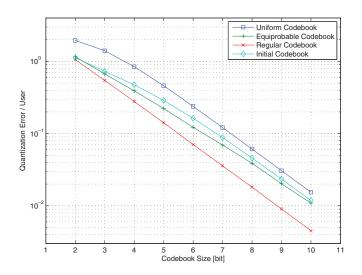
Fig. 2. Comparison of different codebook design approaches for scheduling a user at a later slot. (M = 4, S = 4, SNR = 10 dB, SINR<sub>min</sub> = 7 dB).
