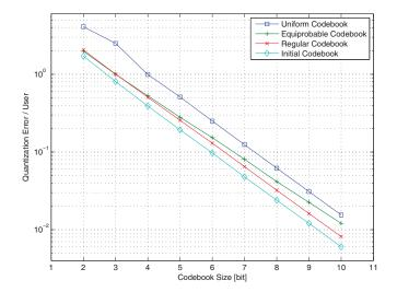
Fig. 1. Comparison of different codebook design approaches for scheduling a user at the first slot.  $(M = 4, |S| = 4, \text{SNR} = 10 \text{ dB}, \text{SINR}_{min} = 7 \text{ dB}).$
