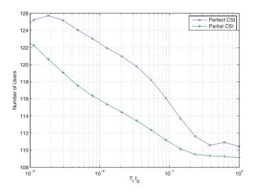
Fig. 5. Average number of users that are scheduled in the same slot as in the previous slot for a varying product of block length  $T_{\rm f}$  and Doppler frequency  $f_{\rm D}$ . (M = 3, K = 100, 150 users, 1000 blocks, Q = 30, SNR = 15 dB, SINR<sub>min</sub> = 5 dB).
