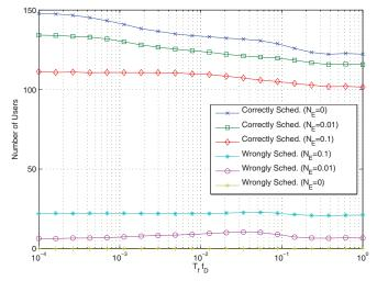
Fig. 6. The effect of erroneous CSI on the number of correctly and wrongly scheduled users in the slot for a varying product of block length  $T_{\rm f}$  and Doppler frequency  $f_{\rm D}$ . (M = 2, K = 100, 150 users, 1000 blocks, Q = 30, SNR = 15 dB, SINR<sub>min</sub> = 5 dB).
