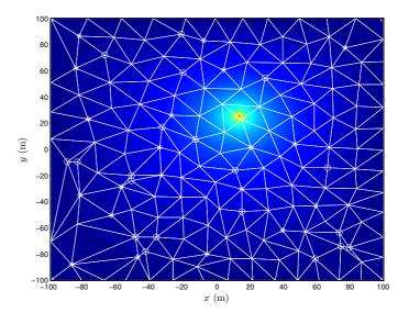
Fig. 1. Contour plot of the simulated field showing a FEM mesh generated for one realization of the random sensor node and POI deployment. A fixed subset of the FEM nodes consists of WSN sensor nodes (o), POIs (\*), and domain corners ( $\Box$ ).
