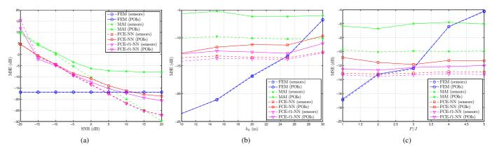
Fig. 2. Comparison of field estimation MSE at sensor node locations (--) and POI locations (-) for different estimation algorithms, plotted vs. (a) SNR of WSN measurements, (b) initial node distance h0 in mesh generation, (c) ratio P/J of number of POIs and sensor nodes.
