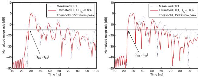
Fig. 9. Example of real measured channel impulse response (CIR) and its estimate using the proposed scheme for different measured positions.
