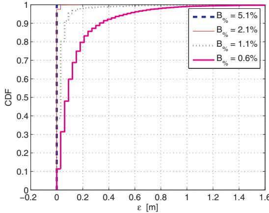
Fig. 6. Range error for different percentage bandwidths.
