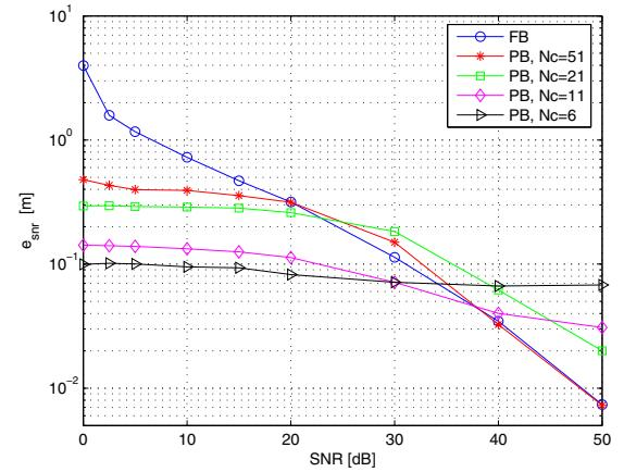
Fig. 8. Effect of SNR on range error for different percentage bandwidths (FB: full band, PB: partial band).
