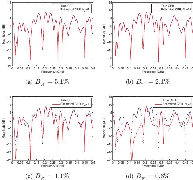
Fig. 4. Comparison between true and estimated UWB channel frequency response (CFR) for different numbers of received sub-bands.
