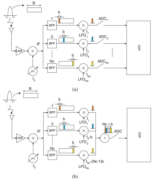
Fig. 1. Proposed receiver scheme based on a) several ADCs b) one ADC. The parameter  $b$  is the width of each sub-band,  $B$  is the bandwidth of the UWB signal and  $N_c$  is the number of received sub-bands.
