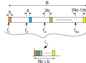
Fig. 2. Illustration of the compression effect using an oscillator with different harmonics.
