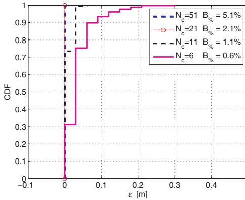
Fig. 10. CDF of range error as a function of  $B_{\%}$  using real measured data.
