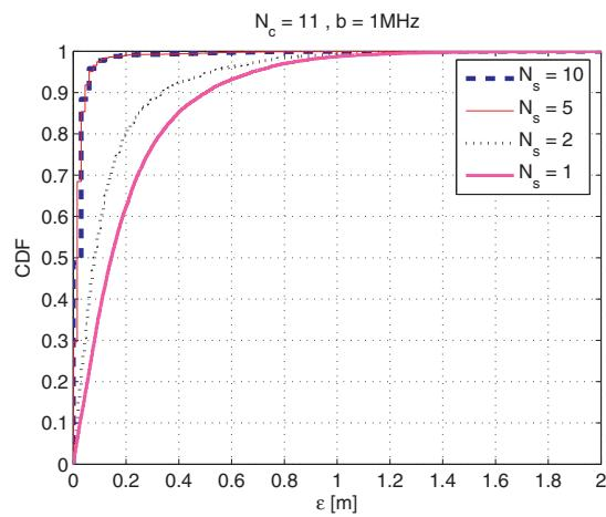
Fig. 7. Effect of the number of samples per sub-band on range error. It should be noted that there is no considerable difference in the results between using a 0.5 or 1 MHz sub-band width because the correlations in an interval of 0.5 or 1 MHz are very similar.
