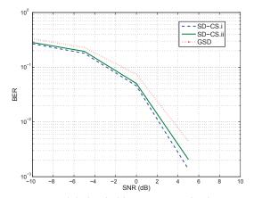
Fig. 2. Demodulation in binary communication: BER.
