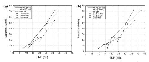
**Fig. 1** Achievable data rates (Mbits/s) as a function of the SNR for a target BER of  $10^{-3}$ (**a**) and  $10^{-4}$ (**b**) for different transmission schemes
