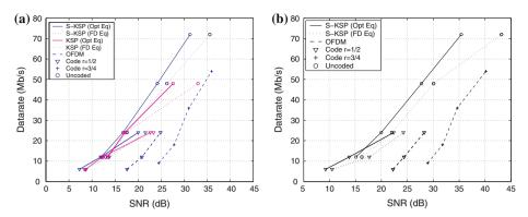
**Fig. 2** Achievable data rates (Mbits/s) as a function of the SNR for a target BER of  $10^{-3}$ (**a**) and  $10^{-4}$ (**b**) for different transmission schemes when realistic channel estimates are considered
