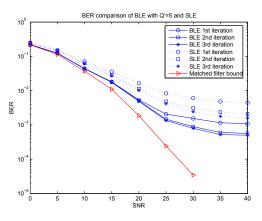
**Fig. 4**. BER comparison of low-complexity block turbo equalizer and SLE
