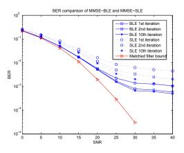
Fig. 3. BER comparison between BLE and SLE
