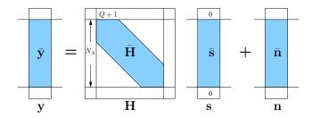
Fig. 1. System input-output relation after removing the guard intervals
