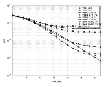
Fig. 6. BER versus SNR for TEQ and PTEQ,  $N_r = 1$  receive antenna.
