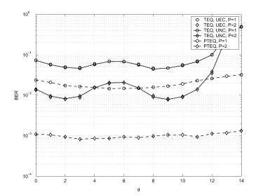
BER versus decision delay d for TEQ and PTEQ,  $N_r = 2$  receive Fig. 8. antennas at SNR = 15 dB
