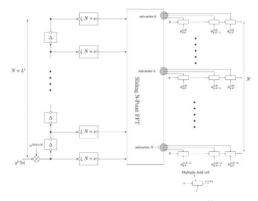
Fig. 4. Sliding FFT of the q'th modulated version of the received sequence  $y^{(r)}[n]$ .
