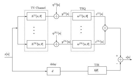
Fig. 3. Block diagram of the TEQ.
