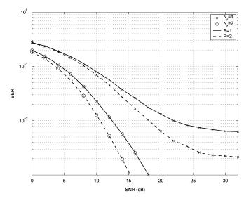
Fig. 9. BER versus SNR for the PTEQ, when the true channel is used to design the equalizer.
