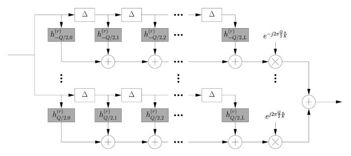
Fig. 2. Block diagram of the BEM realization of a doubly selective channel.
