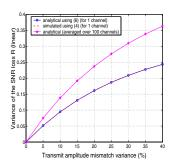
**Fig. 2**. The average (in dB) and the variance (in linear units) of the SNR loss R in the presence of transmit amplitude mismatches
