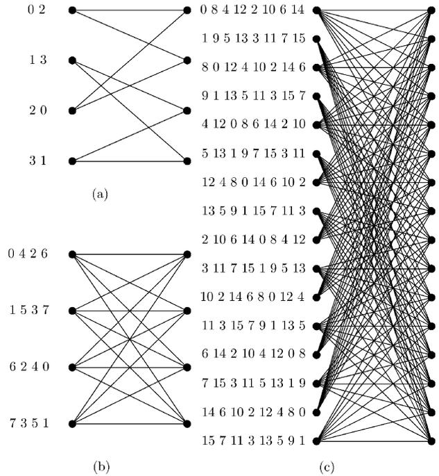
Fig. 3. Three trellis diagrams: (a)  $R = 1/2$  4-state; (b)  $R = 2/3$  4-state; (c)  $R = 3/4$  16-state.
