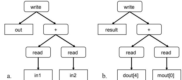
**Figure 7. AST of a) the adder module S and b) the adder module instantiation `*s[4]`.**
