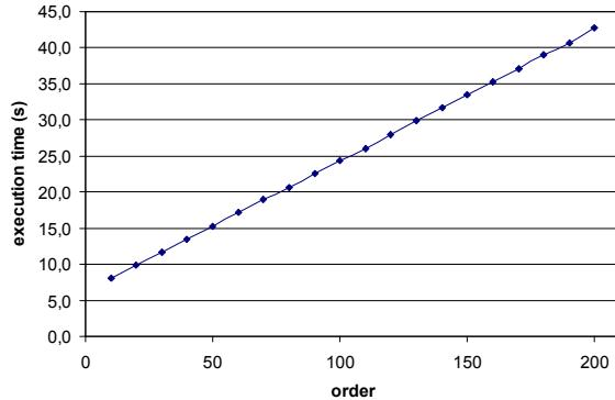
**Figure 8** Execution time of SHaBE for different orders of the FIR filter presented in Figure 2.
