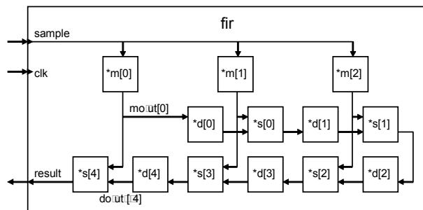
**Figure 5. Dynamically generated hierarchical structure of a 5<sup>th</sup> order filter extracted by SHaBE.**
