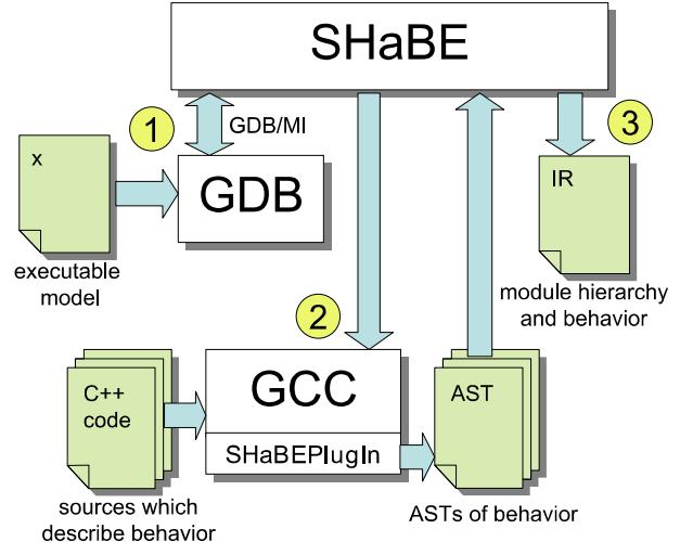
**Figure 1. The architecture of SHaBE (SystemC Hierarchy and Behavior Extractor).**
