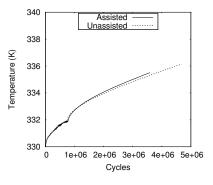
Fig. 10. Comparison of temperature profiles obtained using a conventional data cache (*Unassisted*), and a data cache with an 8-entry assist (*Assisted*).
