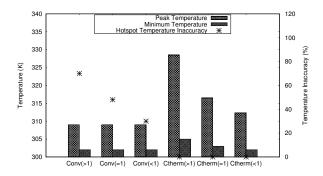
Fig. 7. Comparison of thermal simulation with abstract floorplans (*Conv*) and thermal simulation using Ctherm's fine grained floorplans (*Ctherm*) for a cache memory with varying wordline sharing factor ( $N_{spd}$ ). Three cases:  $N_{spd} > 1$ ,  $N_{spd} = 1$ ,  $N_{spd} < 1$ .
