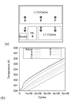
Fig. 11. (a) Floorplan indicating candidate locations for temperature sensors. (b) Tracking from each sensor location.
