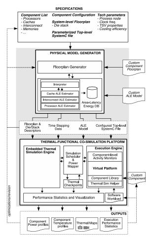
Fig. 1. Ctherm framework for thermal-functional co-simulation
