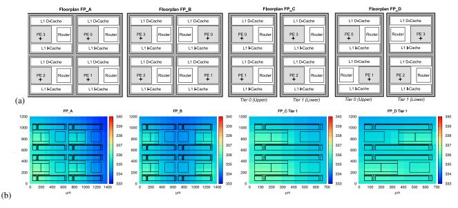
Fig. 9. (a) Floorplan options for the four-PE multiprocessor array. Temperature sensor locations are marked as +. (b) Thermal maps sampled during execution of the *MiBench-dijkstra* workload. Note: Tier 0 is located close to the heatsink/connection to ambient, temperatures are measured in *Kelvin (K)*.
