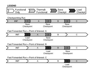
Fig. 6. Illustration of checkpointing run generating thermal checkpoints, followed by fast forwarded runs using saved thermal checkpoints.
