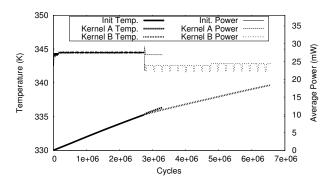
Fig. 12. Temperature and power profiles for initialization, kernel A and kernel B of the extended *first sum* workload
