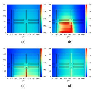
Fig. 8. Heatmaps for 32KB data cache using (a) conventional thermalsimulation with abstracted cache internals, and Ctherm with fine-grained cache floorplans for (b)  $N_{spd} > 1$ , (c)  $N_{spd} = 1$ , (d)  $N_{spd} < 1$ . Temperatures are measured in *Kelvin (K)*.
