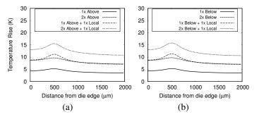
Fig. 6. Influence of stack power density on the actual temperature rise in an observation die. Power sources (a) above observation die (b) below observation die. Note that the case marked +Local uses an active Site 3 heater on the observation die. Each heater dissipates 120mW of power.
