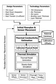
Fig. 1. Thermal characterization flow
