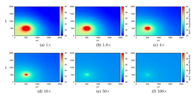
Fig. 3. Thermal map depicting normalized temperature rise across the observation die with increasing effective thermal conductivity relative to conventional silicon  $(1 \times)$ .
