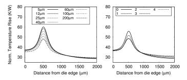
Fig. 5. (a) Influence of varying die thickness on normalized temperature rise. (Thickness of base die:  $250\mu m$ ) (b) Influence of stack depth on normalized temperature rise on an active observation die mounted on a  $250\mu m$  thick base die. (Thickness of observation/stacked dies:  $25\mu m$ )
