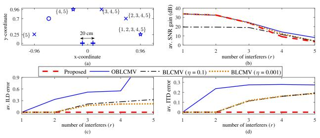
Fig. 1. Locations of sources and microphones (a), average SNR gain over all frequencies and frames (b), average ILD error over all frequencies and all interferers that are present (c), average ITD error over all frequencies and all interferers that are present (d). In (a),  $\star$  and 'x' denote speech shaped white noise and WGN interferers, respectively, 'o' denotes the desired talker source and '+' denote the microphones.
