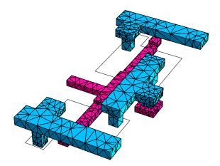
Fig. 6. Mesh for the piecewise linear complex of Figure 5. Note that the whole domain is contained in a rectangular box, which is fully meshed (some tetrahedra have been removed to reveal the contained structure).
