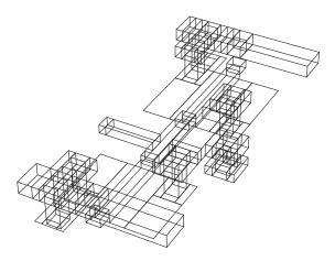
Fig. 4. Original input describing the layout of a cmos-inverter. In the input, faces, segments and nodes are (partially) overlapping.
