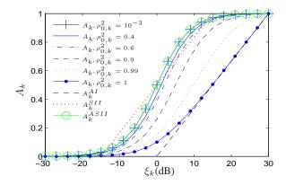
Fig. 1. Comparison of weighting functions.
