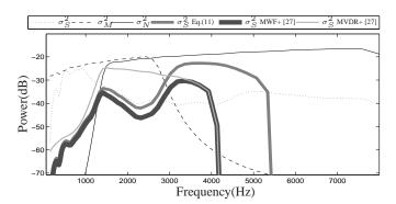
**Fig. 2.** Average spectra for -11.1 dB SNR at the far-end reference microphone and -10 dB SNR at the near-end.
