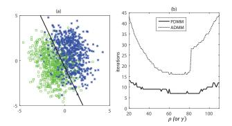
**Fig. 1.** Experimental comparison of PDMM and ADMM in terms of the convergence speed. In subplot (*a*), the samples from the two classes are denoted as (blue) \* and (green)  $\Box$ , respectively. The line in subplot (*a*) represents the global solution ( $\boldsymbol{w}^{\text{glob}}, \boldsymbol{b}^{\text{glob}}$ ). In subplot (*b*), the parameter  $\rho$  (or  $\gamma$ ) was tested for 20, 21, ..., 110.
