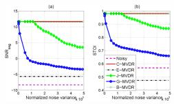
Fig. 5. (a) The  $SNR_{seg}$  of node 1 versus the noise variance. (b) The STOI of node 1 versus the noise variance.
