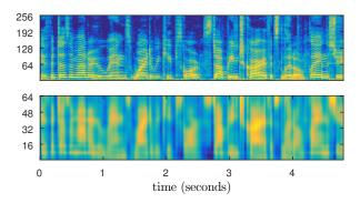
**Fig. 2.** Top: a sequence of log-spectra produced by a talker. Bottom: the same signal projected onto the message articulation space. The bandwidth of the signals is 8 kHz.
