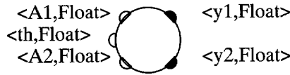
Figure 9.1: Node 'RotRow' with its input and output ports. The labels are the name-type pairs of the ports. All ports have data type 'Float'.
