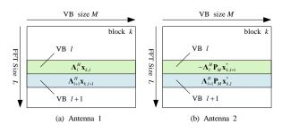
Fig. 3. SFBC V-OFDM transmit block format.
