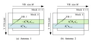
Fig. 2. STBC V-OFDM transmit block format.
