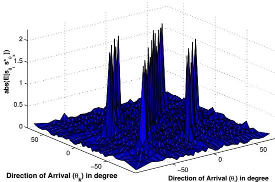
Fig. 3. The magnitude of the elements of the estimated correlation matrix  $\hat{\mathbf{R}}_{\bar{s}}$  computed using LS for the first experiment. Here  $K = 12$ , SNR = 0 dB,  $Q = N = 40$ ,  $L = 28$  and  $M = 10$ .
