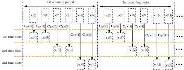
Fig. 1. Illustration of the periodic scanning process where a single scanning period consists of  $L$  time slots. In this example,  $L = 3$  and the number of samples per slot in every antenna is equal to  $S = 2$
