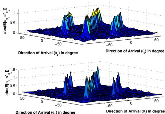
Fig. 5. The magnitude of the elements of the estimated correlation matrices  $\hat{\mathbf{R}}_{\tilde{s}}$  computed using LS (top part) and  $\hat{\mathbf{R}}_{\tilde{s}}$  computed using S-TLS (bottom part) for the second experiment. Here  $K = 12$ ,  $\text{SNR} = 0$  dB,  $Q = 37$ ,  $N = 40$ ,  $L = 28$  and  $M = 10$ .
