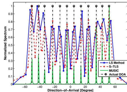
Fig. 4. Normalized spectrum (in normal scale) of LS, S-TLS and MUSIC approaches versus DOA (degree) for the second experiment with  $K = 12$  correlated sources, SNR = 0 dB,  $Q = 37$ ,  $N = 40$ ,  $L = 28$  and  $M = 10$ .
