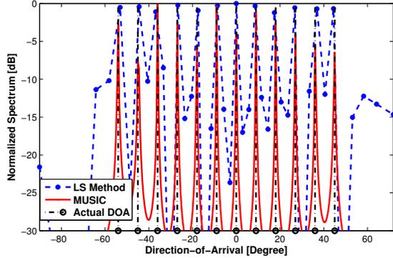
Fig. 2. Normalized spectrum (in dB) of both LS and MUSIC approaches versus DOA (degree) for the first experiment with  $K = 12$  correlated sources, SNR = 0 dB,  $Q = N = 40$ ,  $L = 28$  and  $M = 10$ .
