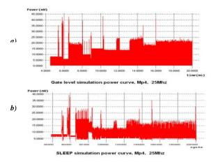
Figure 3. Simulation result of an MP4 decoder. We can observe a similar power profile between Diesel and the SLEEP simulation with a cache power model.
