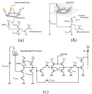
Fig. 2 Schematic diagram of the pixel. (a) Time-resolved fluorescence detection mode. The in-pixel 1bit memory holds the state of the SPAD until next readout cycle. (b) Surface potential detection mode. The digital signal is stored in a 16bit counter outside the pixel array via  $T_{FLIM_N}$  (c) Overall pixel schematic.
