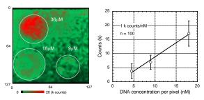
Fig. 5 Two dimensional fluorescence image. The total count rate is increased with increase of Cy5 linked DNA molecules.
