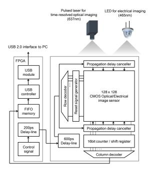
Fig. 1 Block diagram of the system. The time gating control signals are generated by a combination of an on-chip 600ps delay line and an off-chip 200ps delay line.
