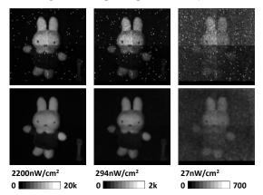
Fig. 4 Optical images under low light illumination. Top: raw image. Bottom: after sensitivity correction and median filtering.
