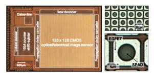
Fig. 3 Microphotograph of the chip. The pixel consists of a SPAD and a donut shaped EGFET gate. The pixel pitch is  $25 \mu m$ .
