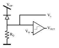
Figure 3. Schematic Diagram of the SPAD and testing electronics. The passive quenching circuit was designed as a ballast resistor. Recharge is achieved passively through the same component. Threshold detection and impedance conversion is implemented via a fast comparator.
