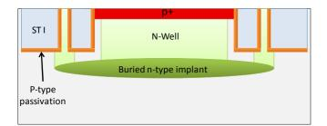
Figure 1. Cross-Section of the circular STI-bound SPAD (not to scale). The STI-interface is passivated using multiple p-type implants, thus reducing the probability of minority carriers entering the multiplication region and triggering dark counts.
