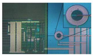
Figure 2. Photomicrogarph of the SPAD and the integrated test electronics implemented in 130nm CMOS technology.
