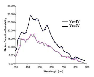
Figure 8. Photon detection probability for two different excess bias voltages.
