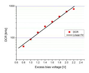
Figure 6. Dark Count Rate at room temperature as a function of the excess bias voltage.
