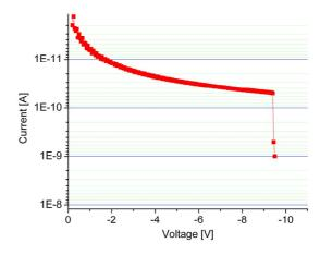
Figure 4. I-V Characteristic of the SPAD.
