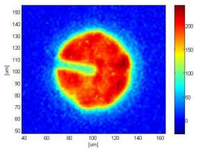
Figure 7. Measurement of the photoemission intensity (arbitrary scale) across the SPAD during avalanche breakdown. Uniform emission indiates equal probability of breakdown on the active area.
