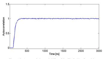
Figure 10. Autocorrelation probability of the SPAD. No afterpulsing contribution could be measured.
