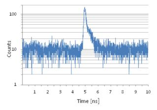
Figure 9. Time response of the SPAD when illuminated by a picosesond light source at 637nm wavelength and 1V of excess bias voltage.
