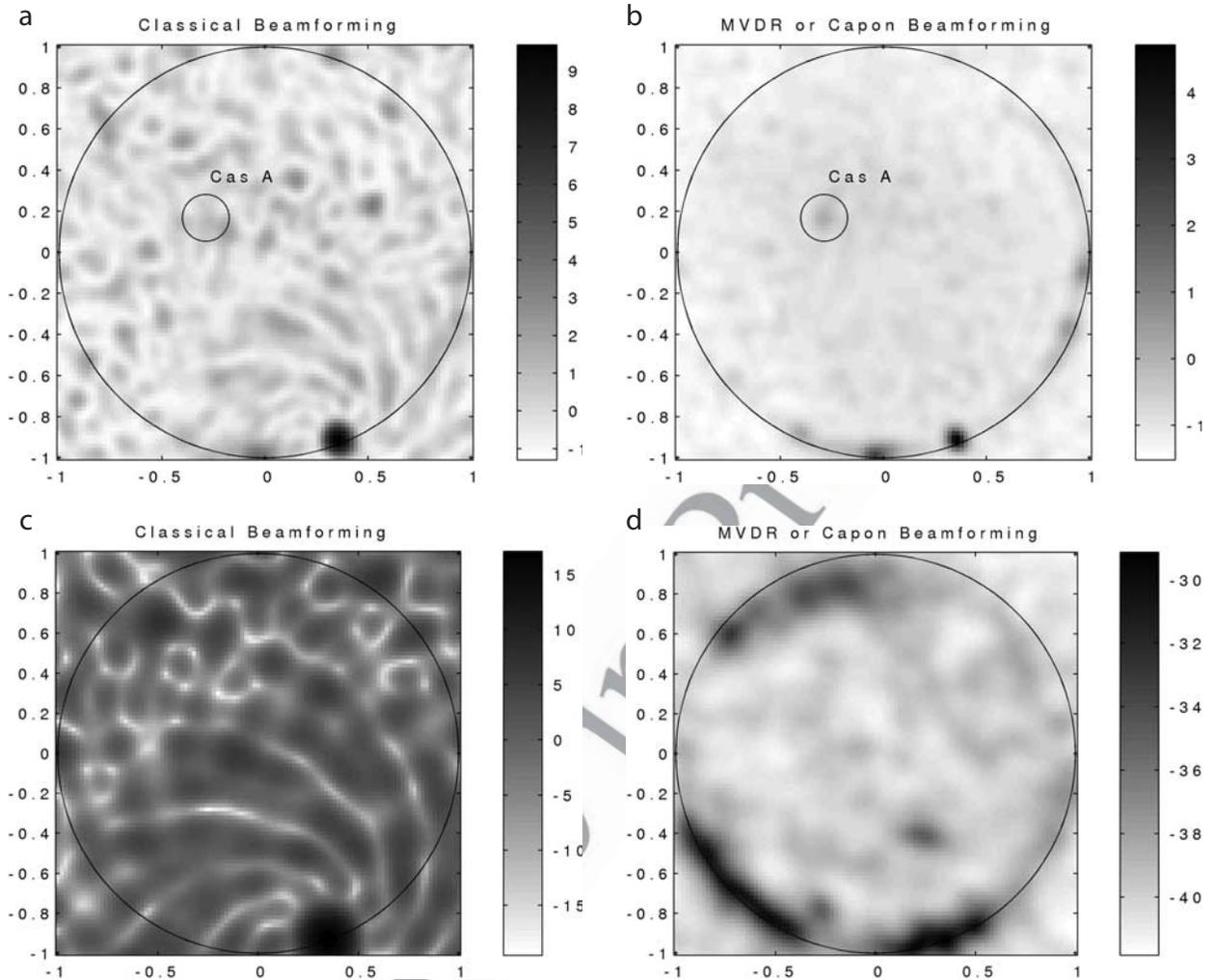
**Figure 9.** Celestial daytime maps obtained with the LOFAR test station using the MVDR beam former and the classical beam former. (a–b) Shown are Cas.A and a transmitter at the horizon at 11.86 MHz and 9.77 kHz bandwidth. (c–d) Shown are the same results, but at a nearby frequency with a more dominant transmitter.
