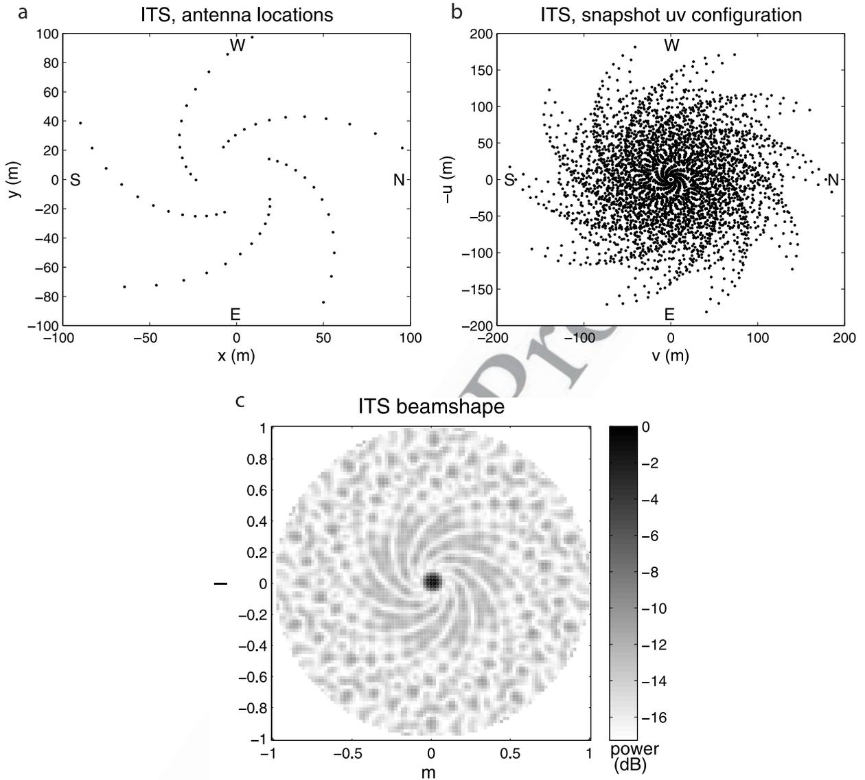
**Figure 2.** (a) LOFAR station ITS antenna configuration, (b) station snapshot ( $u, v$ ) coverage, and (c) station beam shape when the beam is aimed in the zenith direction. The beam shape actually is the response to the entire hemisphere of sky (down to the horizon).
