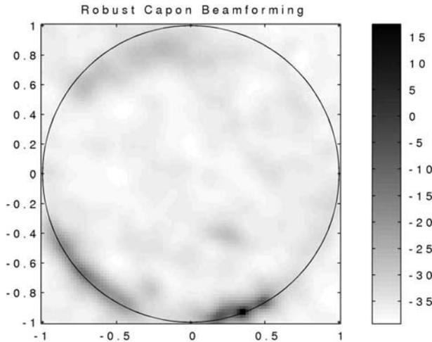
**Figure 10.** Celestial map obtained with the LOFAR test station using the robust capon beam former. The image shows the sky at 11.86 MHz and at a bandwidth of 9.77 kHz. A strong interfering source is visible at the bottom right horizon; a band of interfering signals is visible at the bottom left horizon. Cas.A and the galactic plane are not visible.
