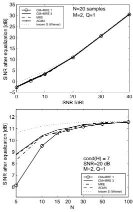
Figure 2. Single user, SINR after equalization
