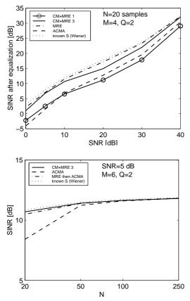
Figure 3. Two users, worst user SINR after equalization
