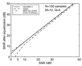
Figure 4. Four users, worst user SINR after equalization
