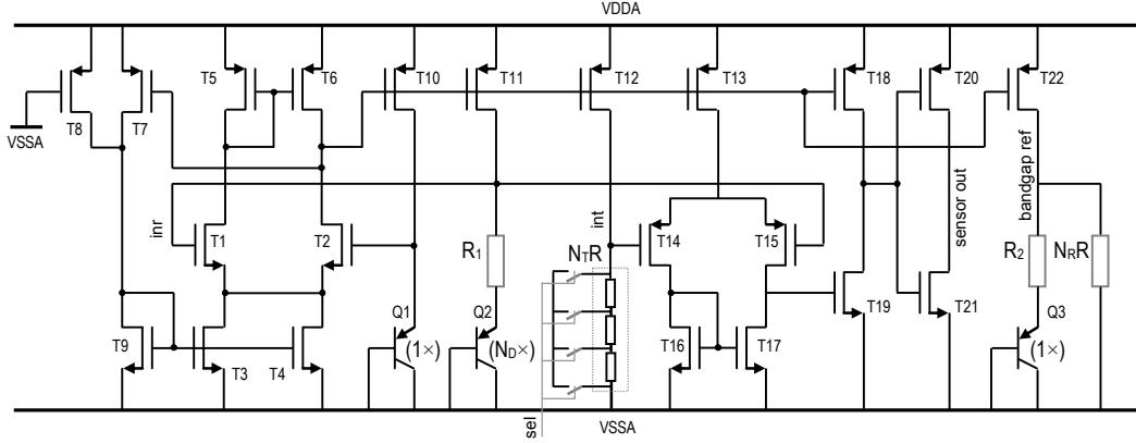
Figure 1: Temperature sensor – schematic view
