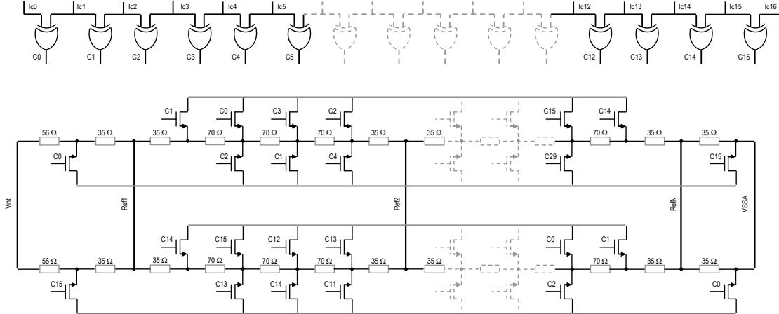
Figure 2:  $N_{TR}$  Resistive network – schematic view
