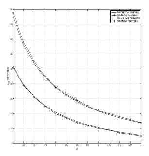
Fig. 4. The value of the scattering radius  $\Delta$  required to obtain a maximum gain equals to half, versus  $\tilde{R}$  (the normalized cluster radius), obtained by numerical calculations and closed-form expressions, for uniform and Gaussian deployments of nodes.
