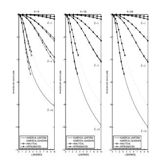
Fig. 3. The maximum gain versus  $\Delta$  for  $N = \{16, 128, 256\}$  and  $\hat{R} = \{1, 4, 16\}$  using numerical calculations, closed-form analytical expressions, and their approximations, for uniform and Gaussian deployments of nodes.
