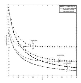
Fig. 5. The 3dB beamwidth versus  $\hat{R}$  (the normalized cluster radius) for  $\Delta = 0.5, 5, 10$  [degrees], with and without local scattering, and for uniform and Gaussian deployments of nodes.
