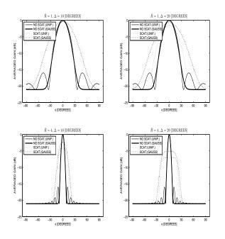
Fig. 2. The averaged gain beampattern for N = 128,  $\overline{R} = \{1, 4\}$ , and  $\Delta = \{10, 20\}$  [degrees] with and without local scattering, and for uniform and Gaussian deployments of nodes.
