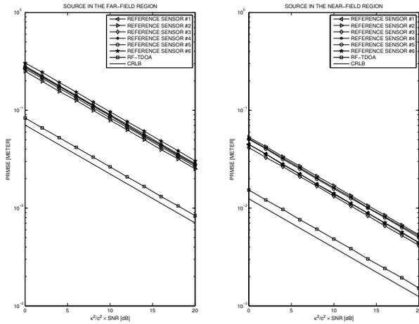
**Fig. 2.** PRMSEs of the proposed method, the method in [7] (for different selections of the reference sensor), and using the CRLB, versus  $\frac{\kappa^2}{c^2}$  SNR given a sensor array with a random configuration.
