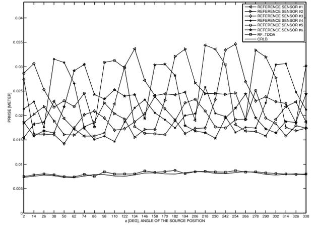
**Fig. 3.** PRMSEs of the proposed method, the method in [7] (for different selections of the reference sensor), and using the CRLB, versus the angle of the source position given a sensor array with a circular configuration.
