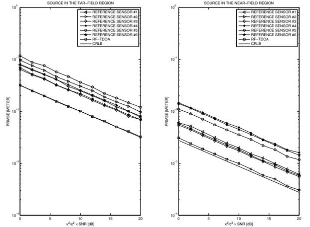
**Fig. 1.** PRMSEs of the proposed method, the method in [7] (for different selections of the reference sensor), and using the CRLB, versus  $\frac{\kappa^2}{c^2}$  SNR given a sensor array with a circular configuration.
