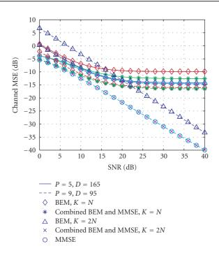
FIGURE 2: MSE versus SNR for D = 165 and D = 95.
