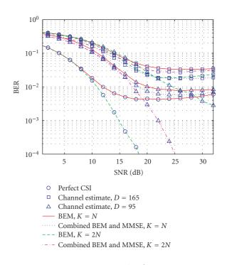
FIGURE 6: BER versus SNR using the MMSE-SDFE.
