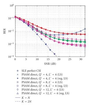
FIGURE 7: BER versus SNR for PSAM-based direct equalization.
