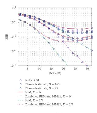
FIGURE 5: BER versus SNR using the MMSE-SLE.
