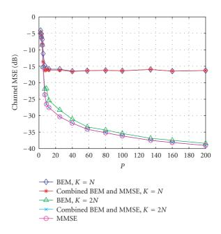
FIGURE 4: MSE channel estimation versus number of pilot symbols P at SNR = 25 dB.
