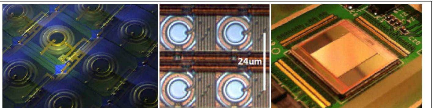
Fig. 1. Artist's rendering of an array of SPADs with optical micro-lenses as light concentrators (left); pixel detail of a high-density large format single-photon imaging sensor fabricated in  $0.35\mu\text{m}$  CMOS technology (center); micro-optical sensor module (right).
