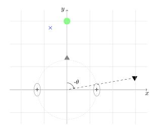
Fig. 1: Typical acoustic scene. The two HA microphones, the assistive microphone, the target signal, and the interferer are indicated by the black "+", the blue " $\times$ ", the green circle, and the black triangle, respectively.
